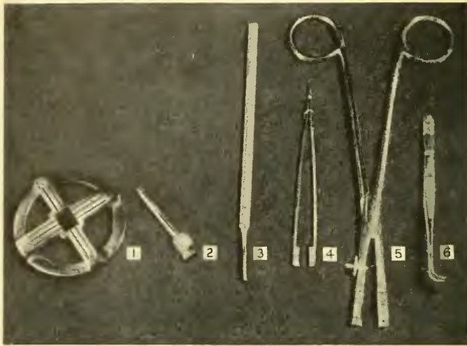
FIG. 11. Convenient tools for the Avena test. 1, frame for dividing agar rectangles into 12 equal blocks with safety razor blade; 2, stamp for cutting the rectangles 8 x 11 mm. from agar disc or sheet 1-2 mm. thick; 3, spatula for application of agar block; 4, cork-tipped forceps for pulling primary leaf loose; 5, decapitation scissors (see Figure 12); 6, forceps for planting in glass holders.
